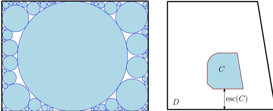
Figure 1: Left: a packing of disks in a rectangle container, where all disks touch the boundary of the container. Right: a convex body  $C$  in the interior of a trapezoid  $D$  at distance  $\text{esc}(C)$  from the boundary of  $D$ . The trapezoid  $D$  is *parallel to*  $C$ : every side of  $D$  is parallel and “corresponds” to a side of  $C$ .
